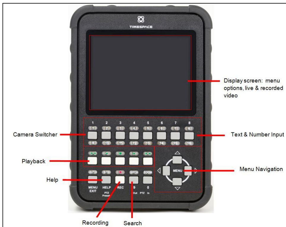
Figure 5 X301 Reviewer/programmer controls
