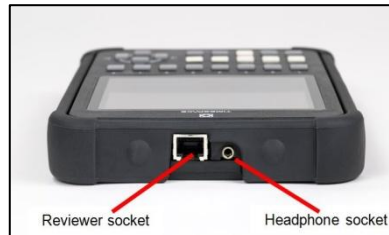
Figure 3 Reviewer socket and headphone connection
